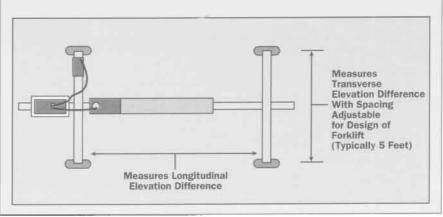
vation from a level plane 10 feet in length. The wheels of most VNA lift trucks are 5 feet apart, requiring a tolerance of 1/16-inch change in elevation. The tolerance is changed to correspond with the lift-truck dimensions.
