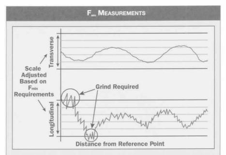
After construction of a defined-traffic concrete floor, the  $F_{\text{min}}$  is not calculated like the  $F_{\text{r}}$  or  $F_{\text{L}}$  measurements of random-traffic areas. The  $F_{\text{min}}$  is actually a direct measurement of the floor surface in the wheel paths of the vehicle for which the defined-traffic area was designed.
