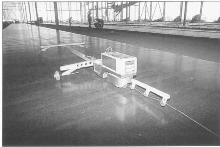
To verify compliance with the minimum superflat requirements in defined-traffic aisles, use a continuous-recording floor profilometer configured to run in the traffic wheel tracks. Do not use equipment designed to measure random-traffic areas.
